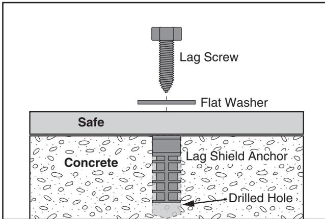
Installation of lag shield anchors requires you to drill holes into the concrete. Drilling into concrete properly requires a hammer drill with an appropriate sized concrete drill bit.
