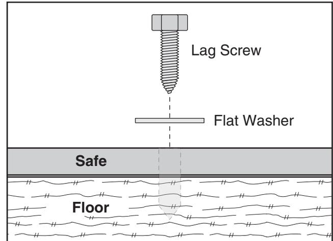
Installation of lag screws works best if holes are pre-drilled to accommodate the lag screws. A standard handheld power drill with the appropriate-sized wood drill bit is required to complete the job.
