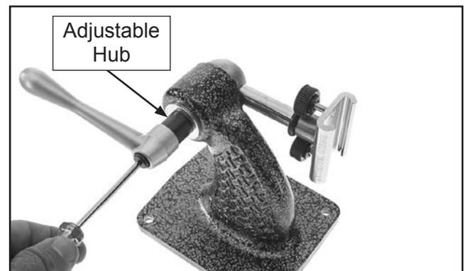
Figure 5. Installing lock handle onto base.
