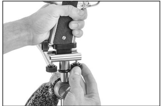
**Figure 12.** Securing firearm in vise.
