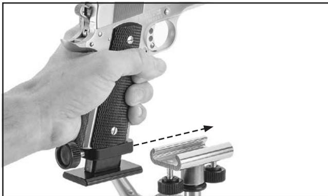
**Figure 11.** Aligning firearm mounted on magazine holder with dovetail mount.
