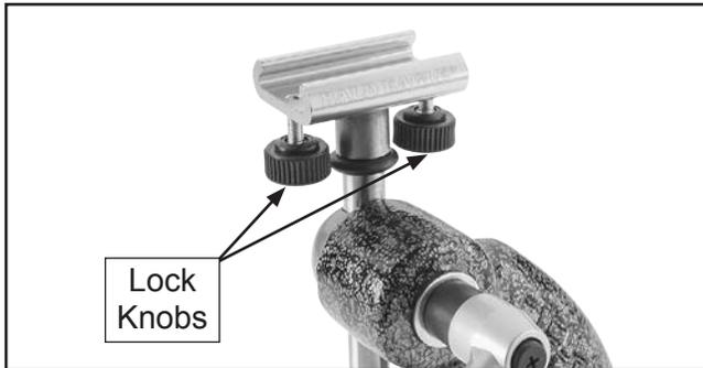
**Figure 10.** Location of dovetail mount lock knobs.
