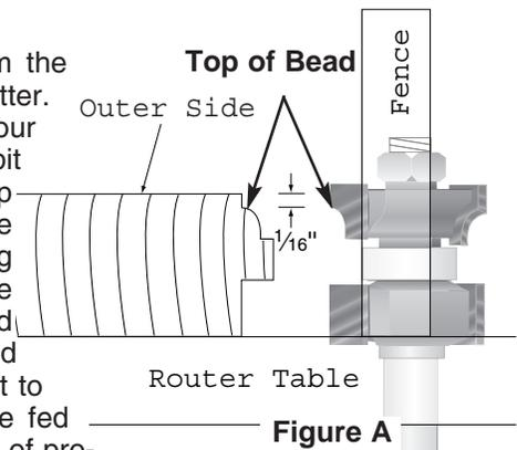
Run all of the stiles and rails for the project through the cutter before changing bits to do the rail ends.
