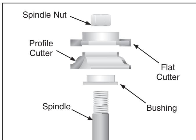
**Figure C.** Set-up for cutting stiles.
