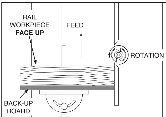
**Figure B.** Cutting the ends of rails.
