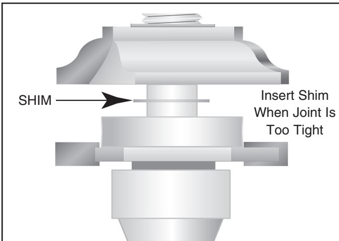
**Figure E.** Adjustment to fit panel.
