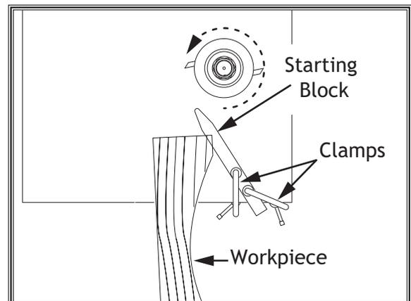
**Figure 8.** Typical setup for performing irregular shaping.
