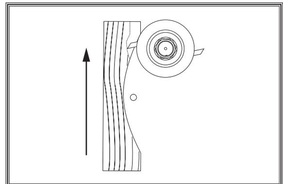
**Figure 11.** Feeding workpiece against moulding head knife.
