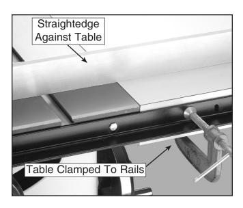
**Step 11.** Attach the rails to the table with the (8) <sup>3</sup>/<sub>8</sub>"-16 x 1<sup>3</sup>/<sub>4</sub>" hex bolts, (16) <sup>3</sup>/<sub>8</sub>" washers and (8) <sup>3</sup>/<sub>8</sub>"-16 nuts. The assembly order should be hex bolt, flat washer, rail, extension table, flat washer, and hex nut. *Note—some assemblies will require* <sup>3</sup>/<sub>8</sub>" holes drilled through the table to match fence rail holes for mounting.
