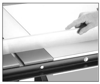
**Step 13.** Mount the fence to the rails, and slide the fence back and forth to ensure proper operation.
