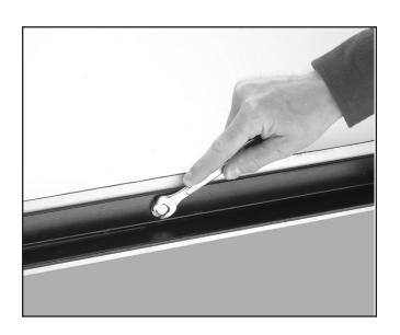
**Step 12.** Use the straightedge to verify that the extension table is flush with the saw table and is even along its entire length. Minor adjustments may be made by adjusting the rail-to-table hex bolts or by rotating the feet. Note—lock the ½"-12 hex nuts to keep the feet in place after adjustments are final.
