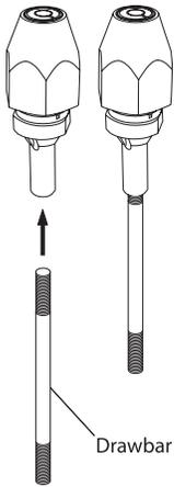
Completely thread the drawbar up and into the router bit spindle approximately 10-15 turns until the drawbar is tight.
