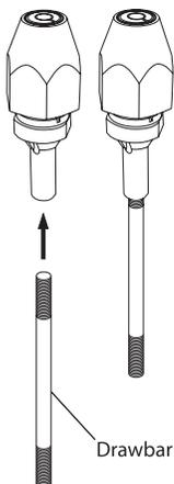
Completely thread the drawbar up and into the router bit spindle approximately 10-15 turns until the drawbar is tight.
