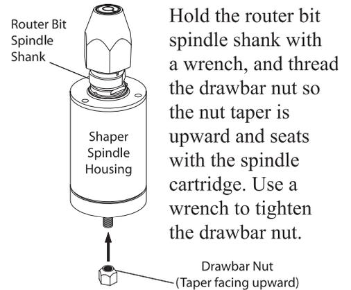
Hold the router bit spindle shank with a wrench, and thread the drawbar nut so the nut taper is upward and seats with the spindle cartridge. Use a wrench to tighten the drawbar nut.
