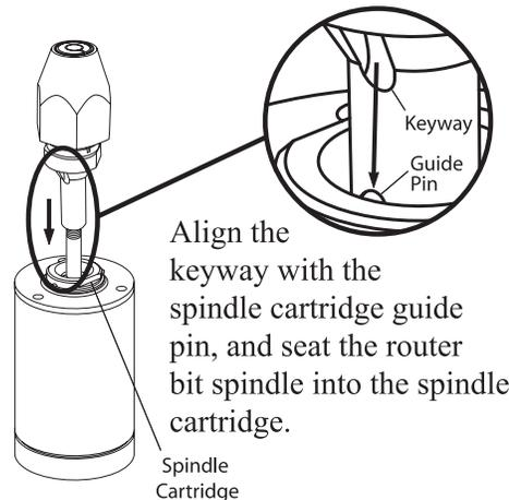
Align the keyway with the spindle cartridge guide pin, and seat the router bit spindle into the spindle cartridge.
