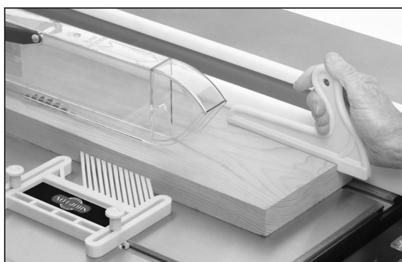
Figure 2. Using the push block.
