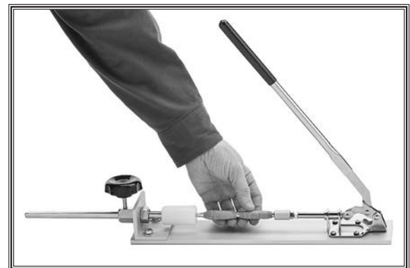
Figure 8. Holding pen steady during assembly operation.
