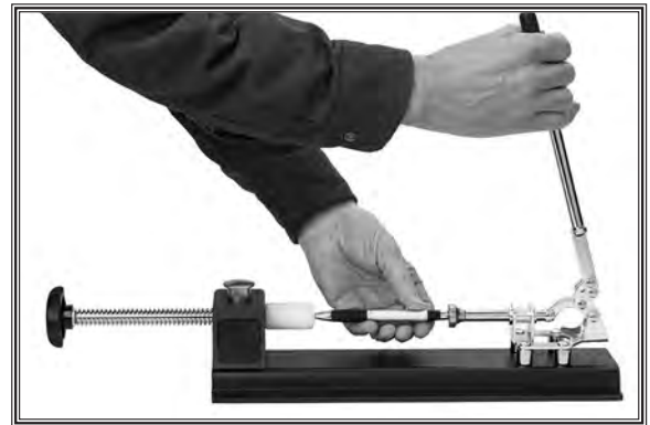
Figure 8. Holding pen steady during assembly operation.
