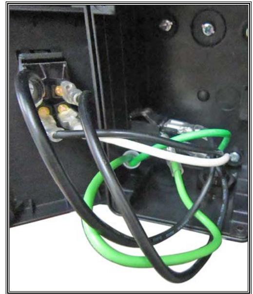
Figure 13. ON/OFF switch and 110V outlet wiring.
