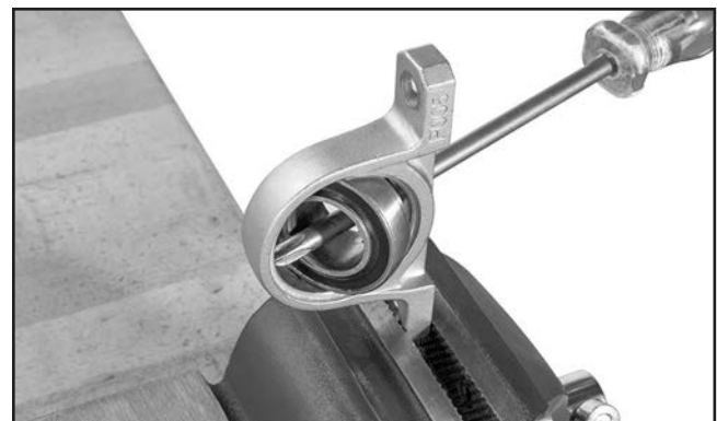
Figure 71. Leveraging bearing into housing.
