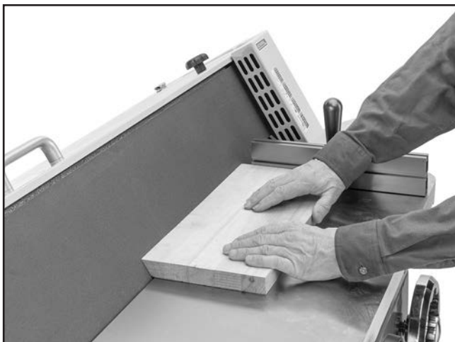
Figure 55. Typical bevel sanding operation.
