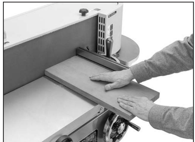
Figure 54. Typical end sanding operation.
