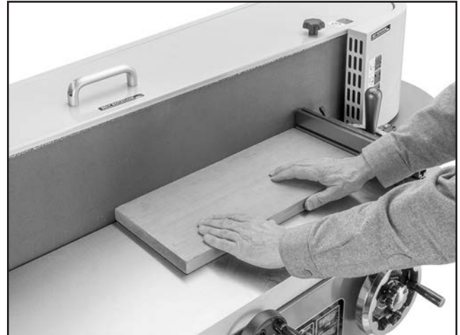
Figure 53. Typical edge sanding operation.
