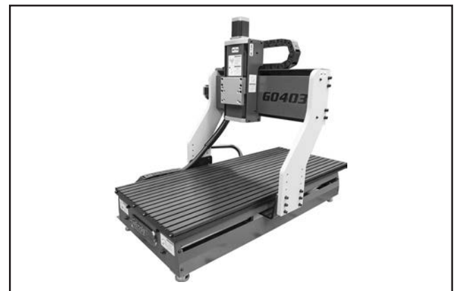
Figure 40. Gantry in raised position.
