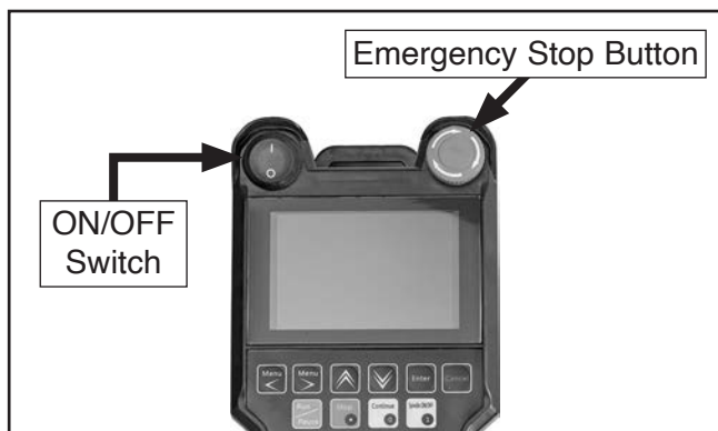
Figure 15. Location of DSP controller power controls.
