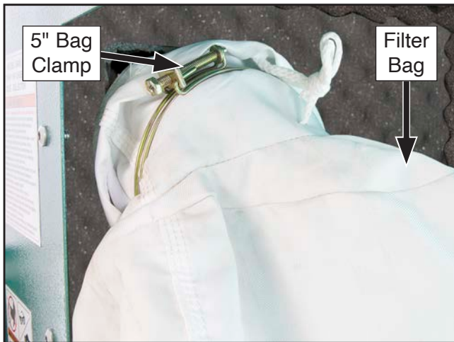
Figure 17. Filter bag secured to dust port outlet.
