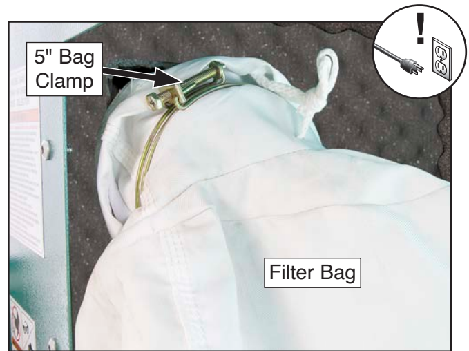
Figure 41. Filter bag removal components.
