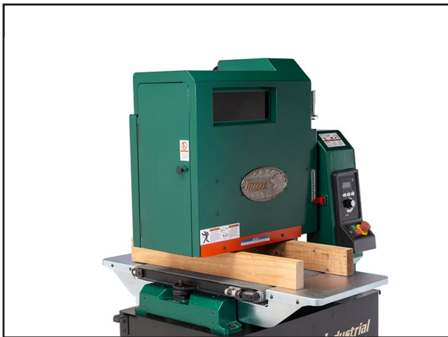
Figure 46. Example of gauge blocks placed under drum.
