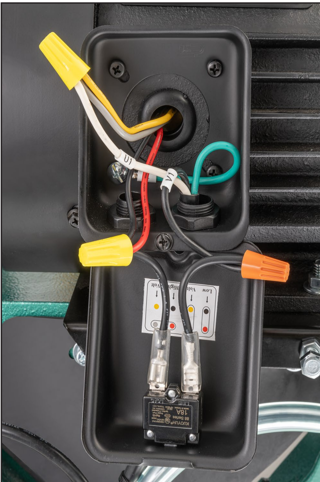
Figure 94. Main motor wiring (115V).
