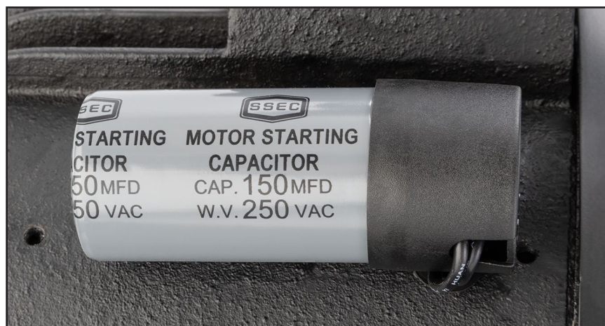
Figure 98. Motor start capacitor wiring.
