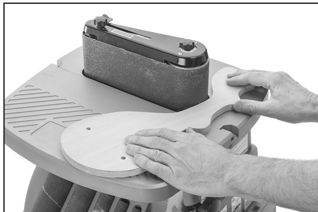
Figure 30. Example of edge sanding inside curve.
