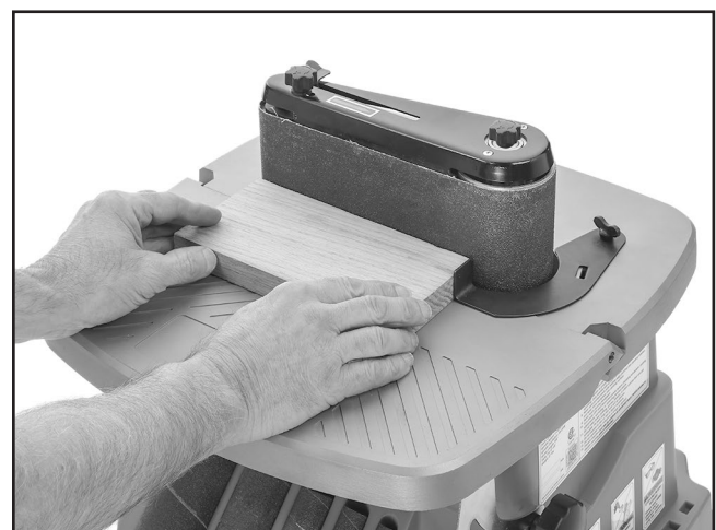
Figure 28. Example of using backstop to edge sand workpiece against platen.
