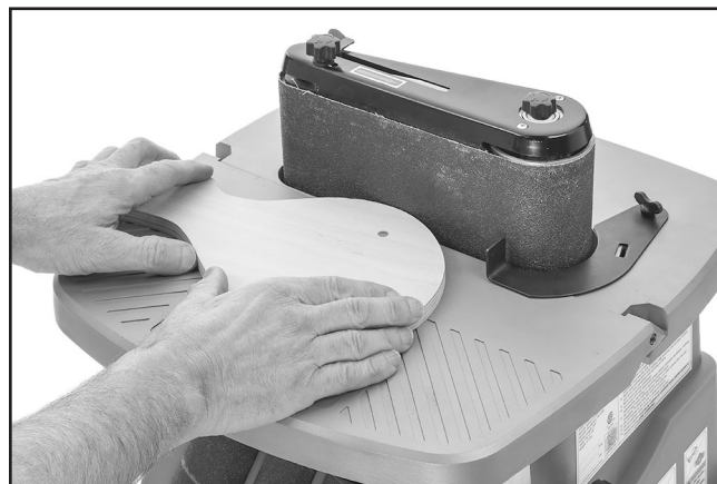
Figure 32. Example of sanding outside curve with edge sanding attachment.
