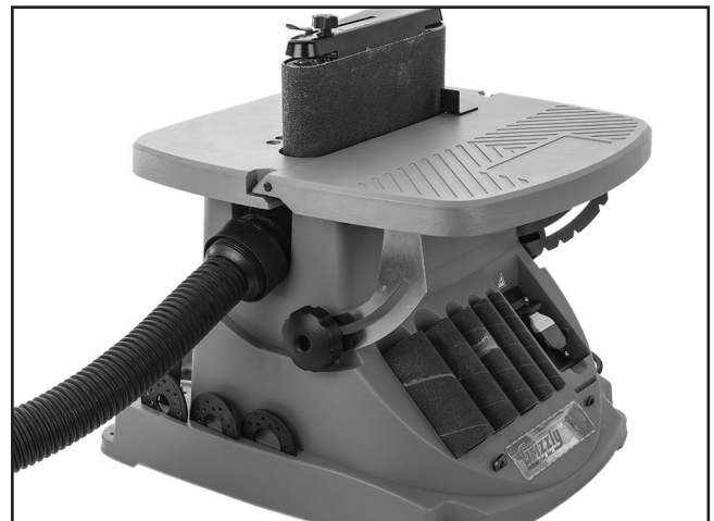
Figure 14. Example of dust hose attached to dust port.
