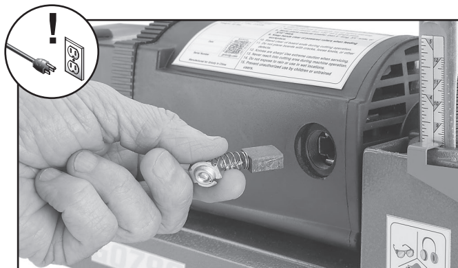
Figure 28. Example of removing motor brush.
