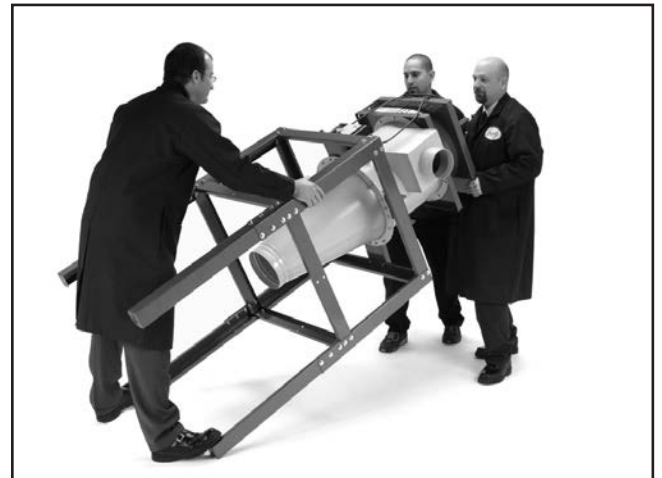
Figure 13. Lifting the assembly upright.
