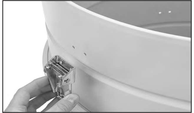
Figure 24. Installing drum latches on collector drum.
