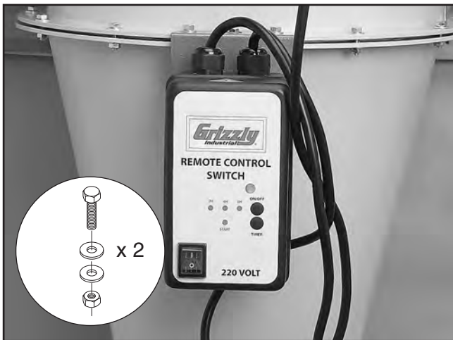
Figure 31. Magnetic switch mounted to funnel.
