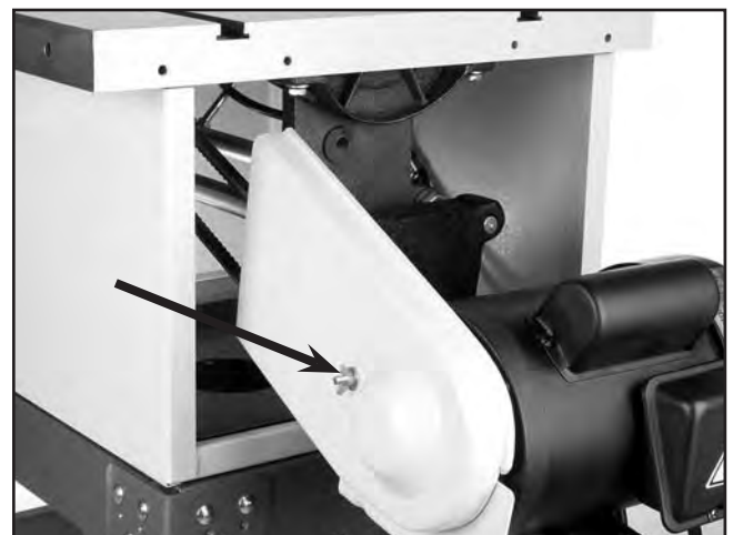
Figure 23. Installed V-belt guard cover.
