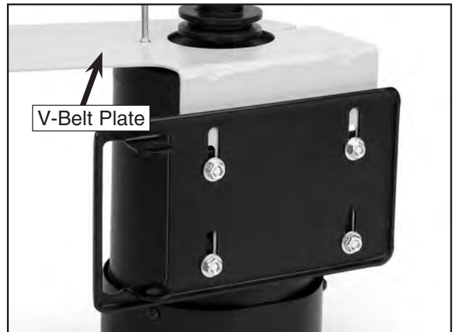
Figure 18. Installed V-belt plate.
