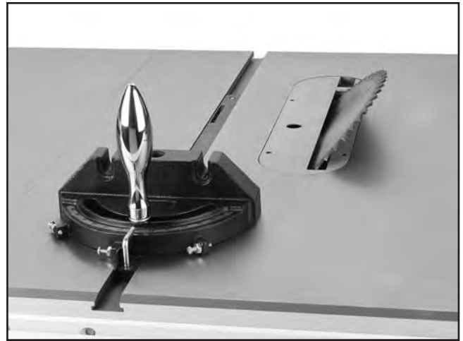
Figure 47. Blade tilted to 45° (guard removed for clarity).
