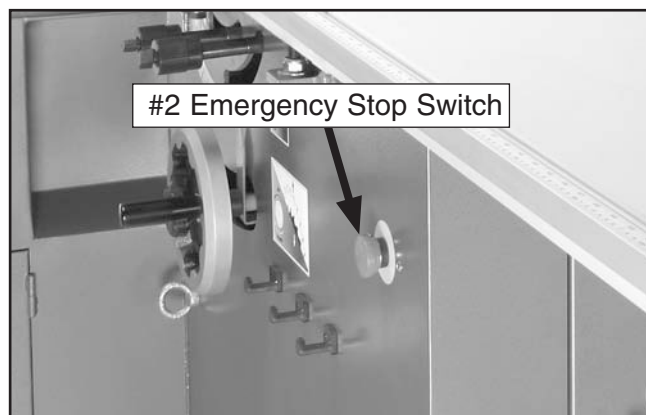
Figure 54. Emergency stop switch #2.
