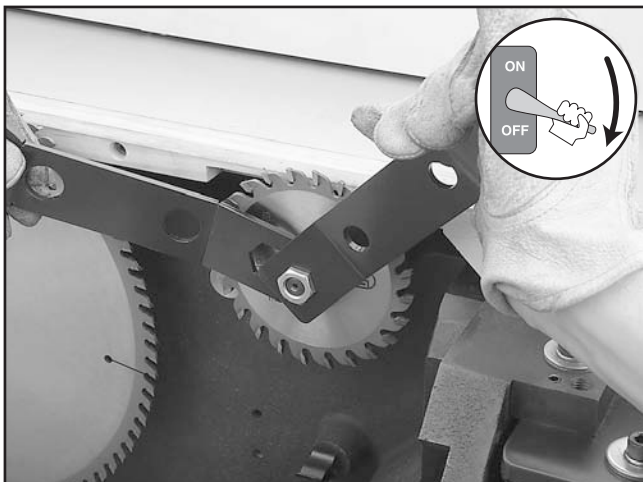
Figure 71. Removing the scoring blade.
