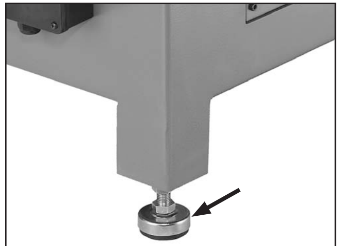
Figure 19. Foot studs placed in base feet.
