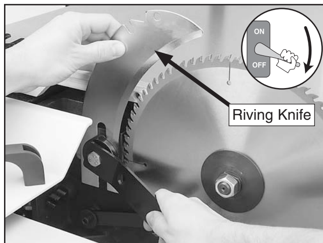
Figure 36. Installing the riving knife.
