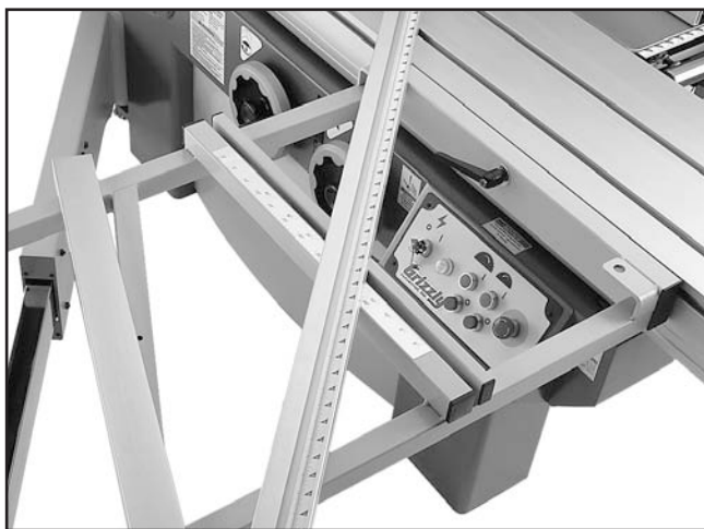
Figure 85. Fence set-up for 90° to 135° cuts.
