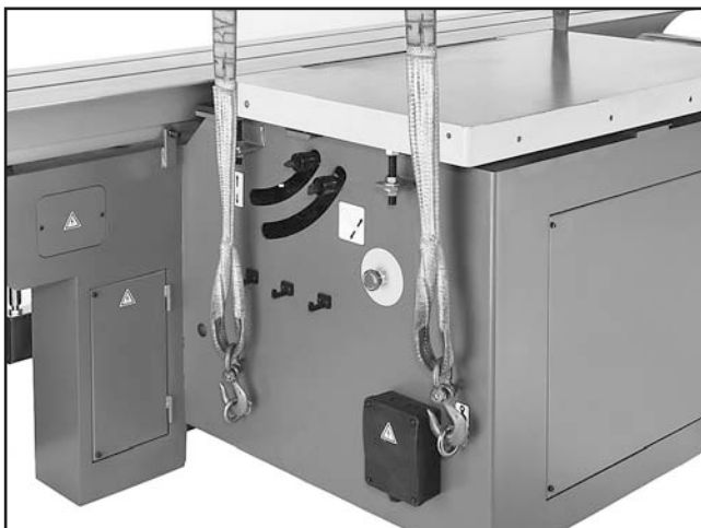
Figure 18. Lifting the saw base unit.
