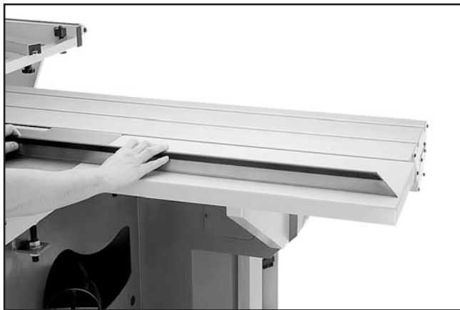
Figure 25. Checking with a straightedge.
