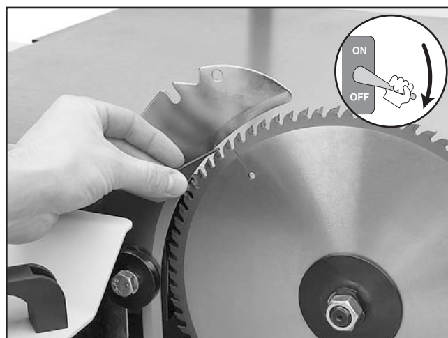
Figure 37. Adjusting the riving knife.
