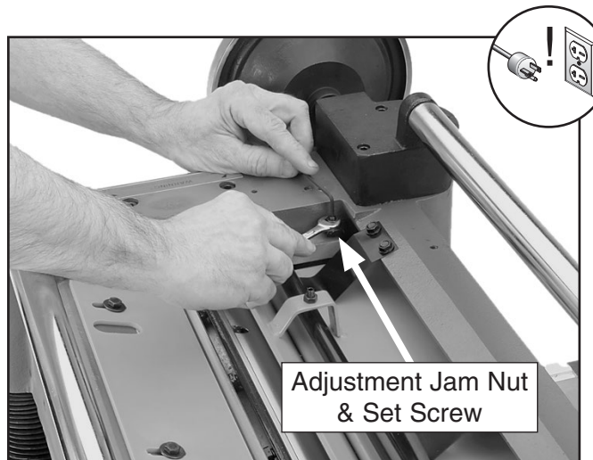
Figure 66. Example of adjusting the pressure bar height.
