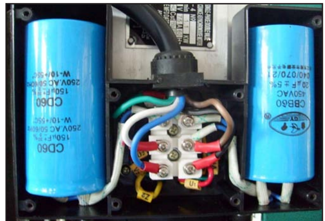
Figure 37. Spindle motor capacitors and wiring connections.
