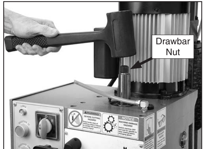
Figure 14. Unseating the arbor/cutter.
