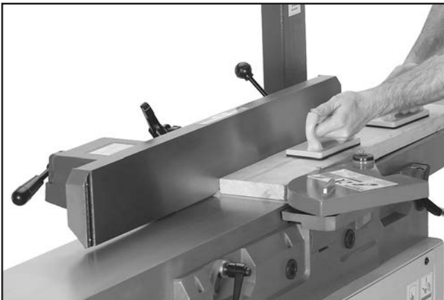
Figure 31. Example of surface planing operations.
