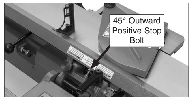
Figure 66. Adjusting fence 45° outward.
