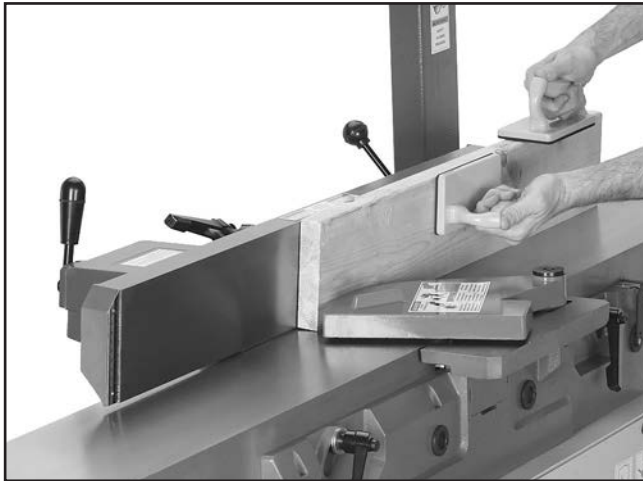
Figure 33. Example of edge jointing operation.
