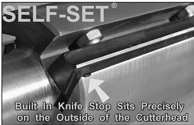
Figure 39. Dispoz-A-Blade® Holder and Knife.
