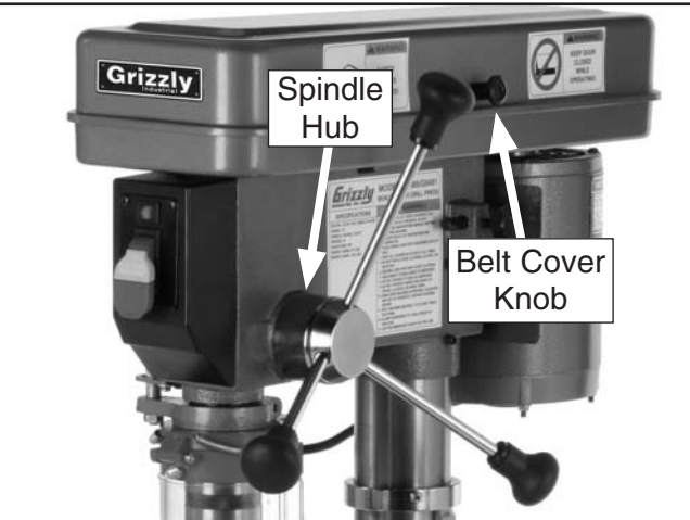
Figure 18. Downfeed handles and belt cover knob installed.
