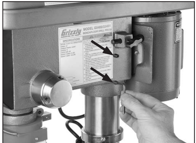
Figure 13. Securing headstock to column.
