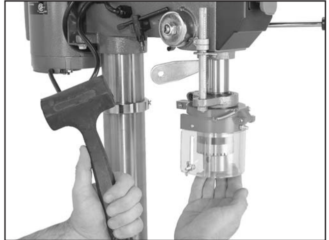
Figure 32. Using drift key to remove arbor.
