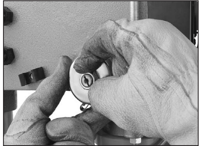
Figure 42. Loosening cover nut.
