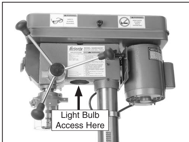
Figure 20. Light bulb access location.
