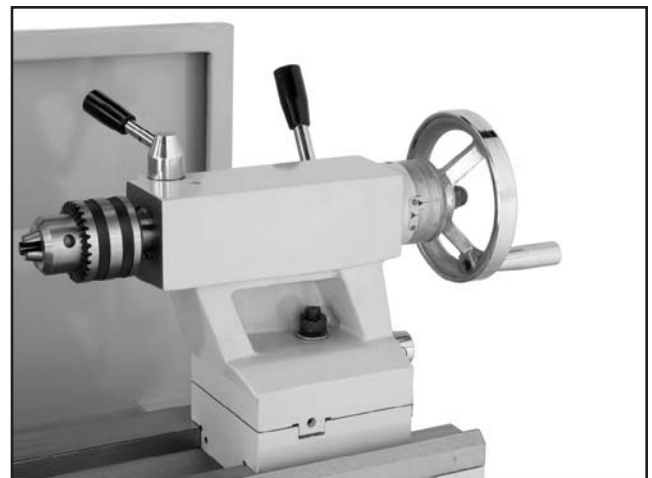
Figure 18. Setting up tailstock for drilling.
