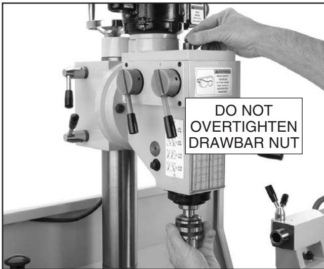
Figure 44. Aligning drawbar with chuck arbor.
