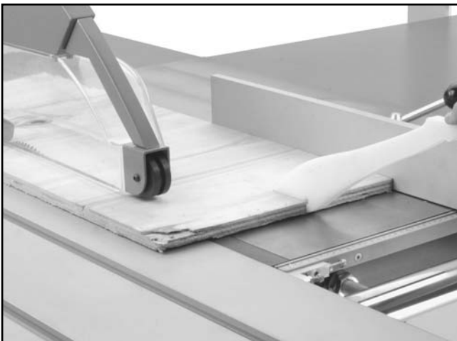
Figure 66. Rip cutting using the traditional table saw technique.
