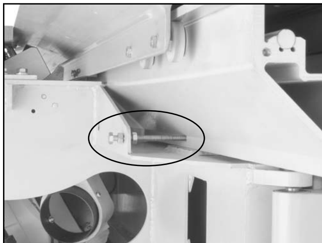
Figure 55. Sliding table parallel adjustment bolt (other side not shown).
