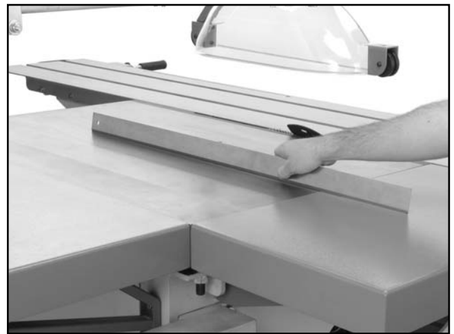
Figure 40. Checking with a straight edge.
