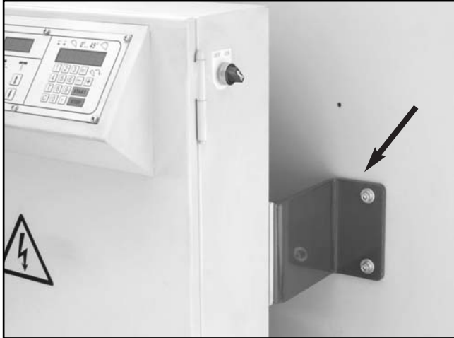
Figure 21. Control panel shipping brace.
