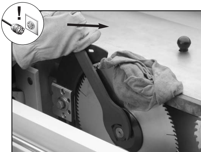
Figure 82. Removing arbor nut to change blade.
