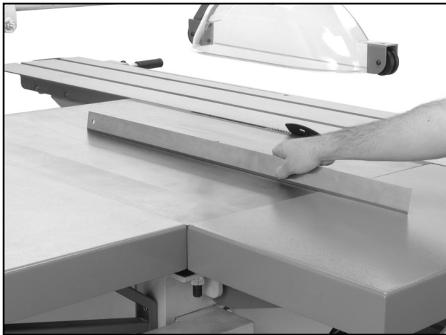
Figure 7. Checking the table surfaces with a straightedge.
