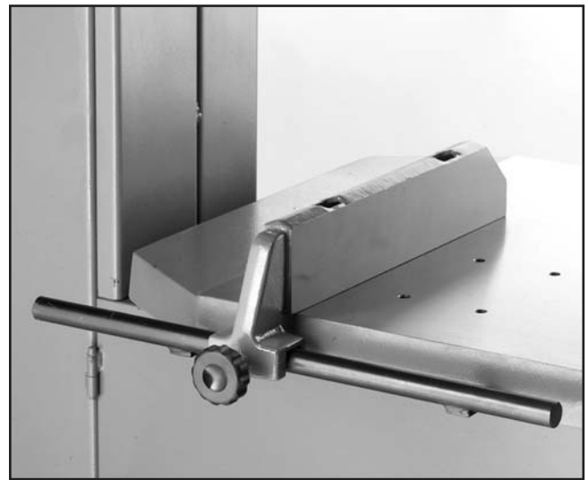
Figure 7. Fence mounted on rail.
