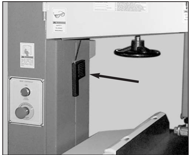
Figure 22. Blade tension gauge.
