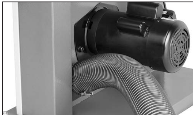
Figure 34. Dust hose attached to bottom dust port.
