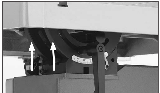
Figure 95. Trunnion lubrication location (G0514X2/G0514X2B/G0514X3).
