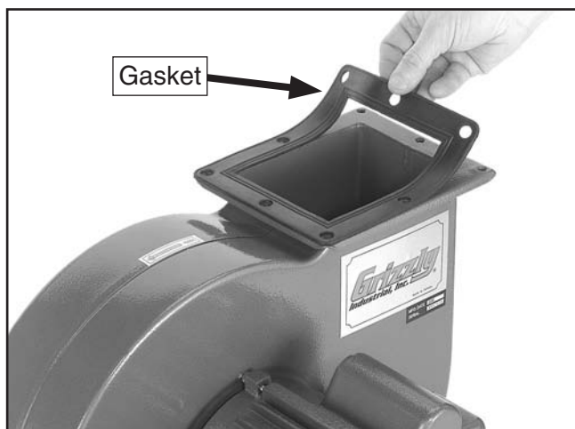
Figure 13. Positioning impeller outlet gasket.
