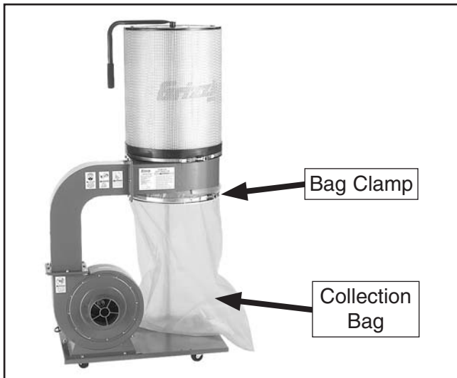
Figure 21. Collection bag installed.
