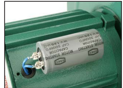
Figure 70. G0548Z start capacitor.
