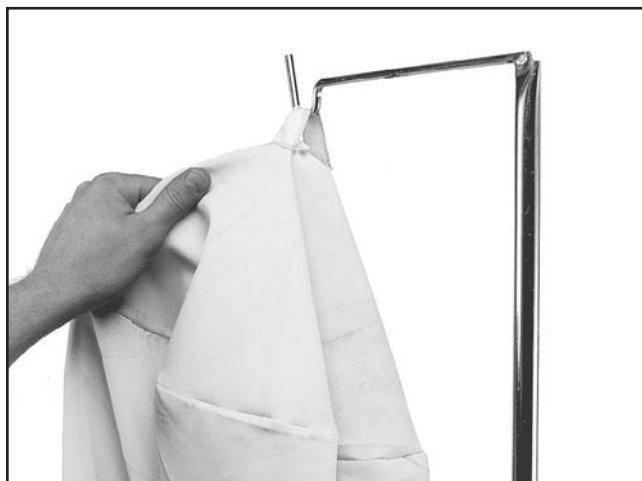
Figure 32. Attaching upper filter bag.
