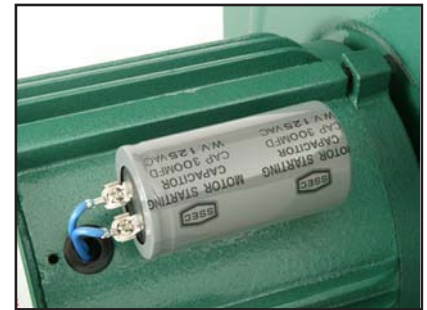
Figure 74. G1029Z2 start capacitor.
