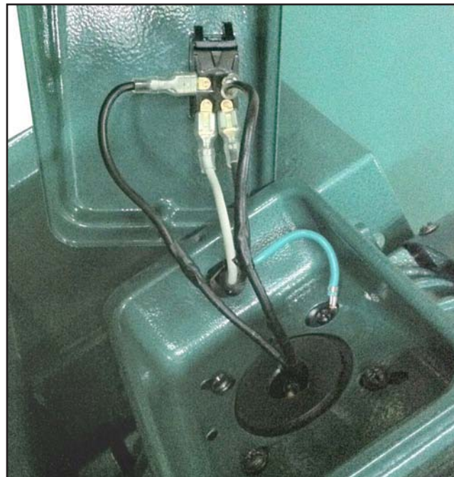
Figure 75. G1029Z2 junction box and switch.
