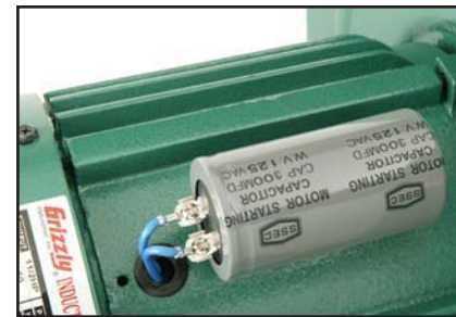
Figure 72. G1028Z2 start capacitor.
