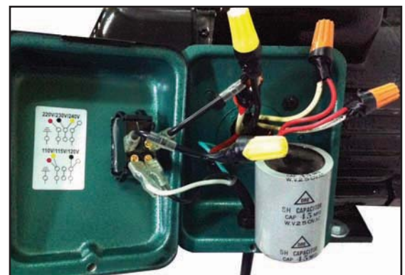
Figure 73. G1028Z2 junction box, switch and run capacitor at 120V.
