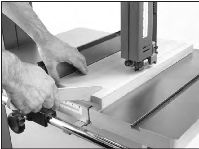
Figure 31. Ripping with a push stick.
