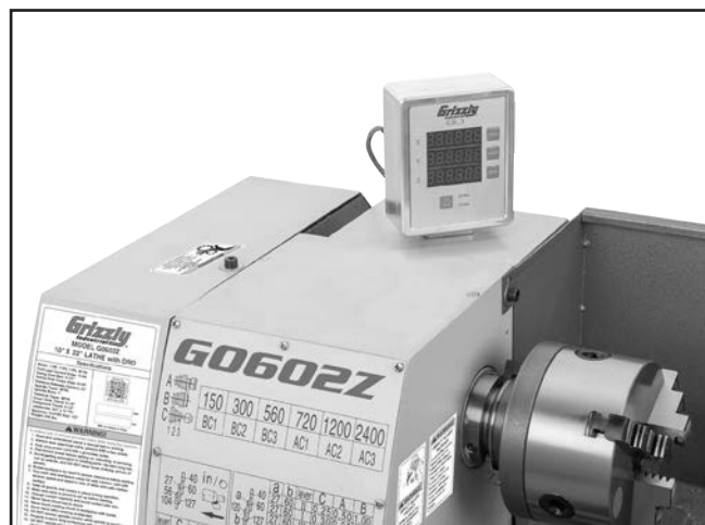
Figure 9. DRO magnetically mounted on lathe headstock.
