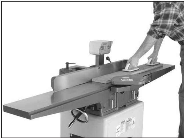
Figure 22. Typical surface planing operation.
