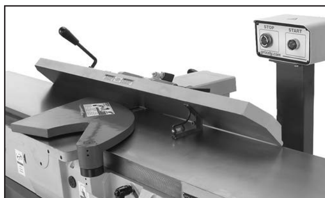
Figure 57. Fence adjusted 45° inward.
