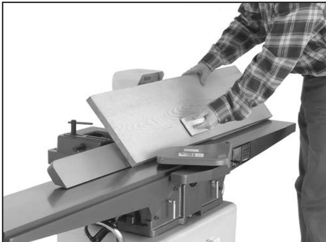
Figure 26. Typical bevel cutting operation.
