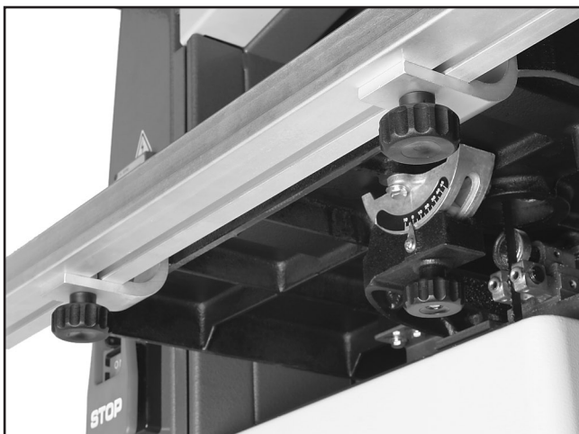
Figure 10. Fastening front fence rail.
