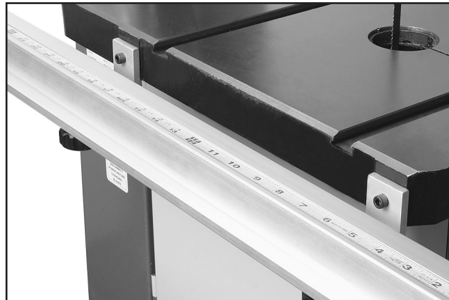
Figure 15. Scale installed on front fence rail.
