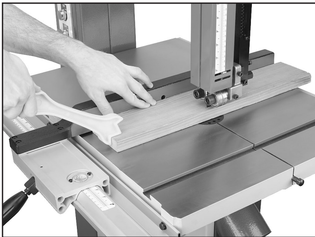
Figure 32. Typical ripping operation.
