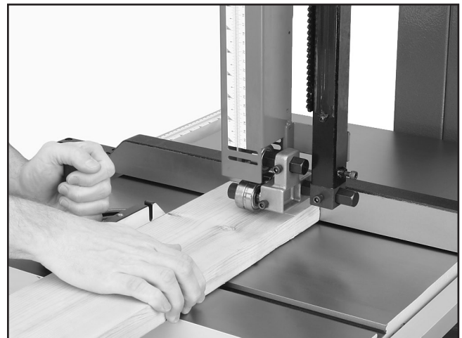
Figure 33. Typical crosscutting operation.
