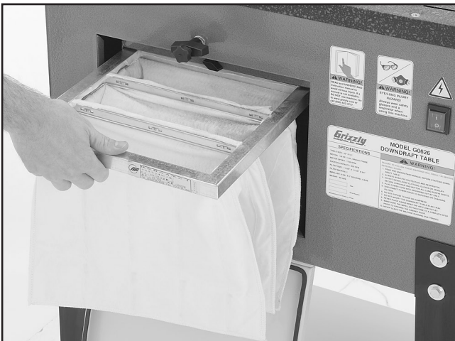
Figure 8. Installing filter bag.
