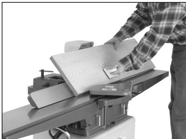
Figure 36. Typical bevel cutting operation.
