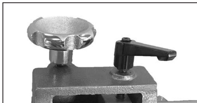
Figure 3. Lock lever installed.
