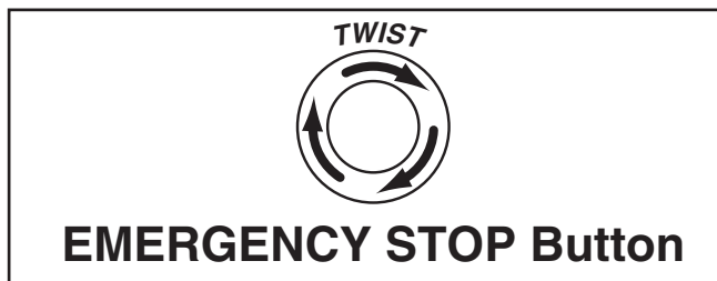
Figure 15. Resetting the EMERGENCY STOP switch.
