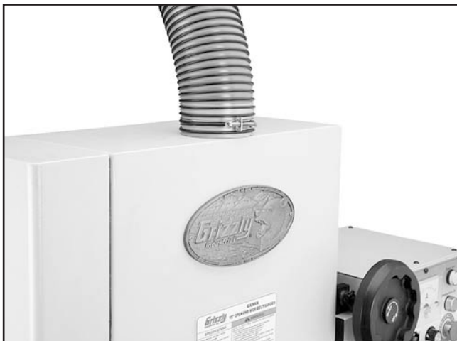
Figure 14. Dust hose attached to dust port.
