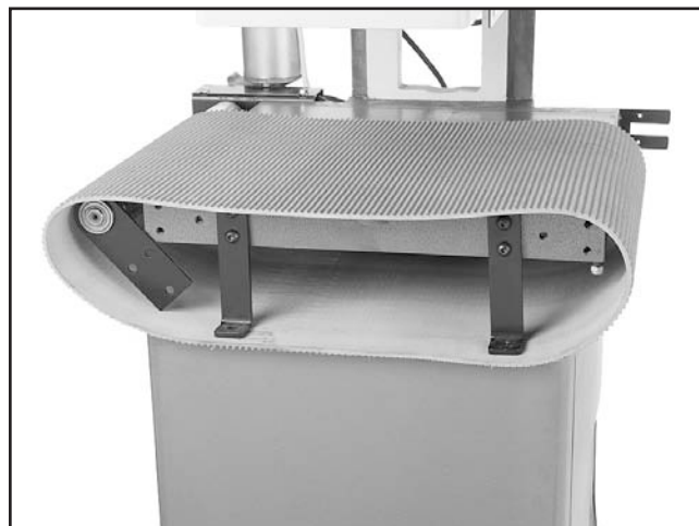
Figure 44. Conveyor belt partially removed from the sander.
