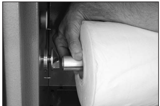
Figure 29. Removing recovery axle.
