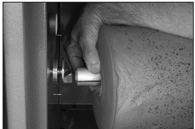
Figure 25. Removing recovery axle.
