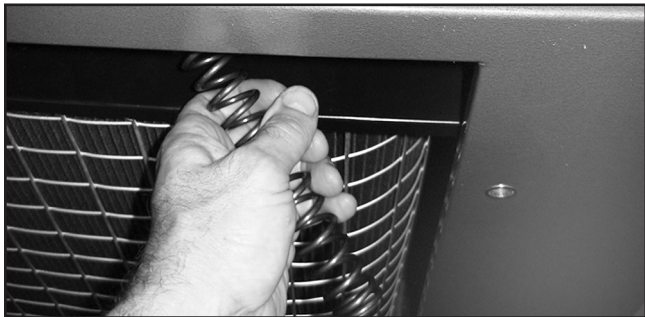
Figure 34. Removing vibration filter spring.
