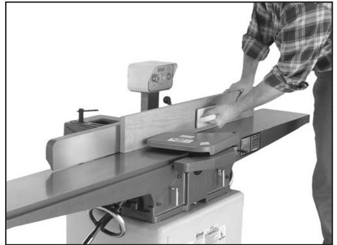
Figure 28. Typical edge jointing operation.
