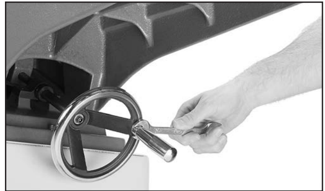
Figure 12. Securing the handwheel handle.
