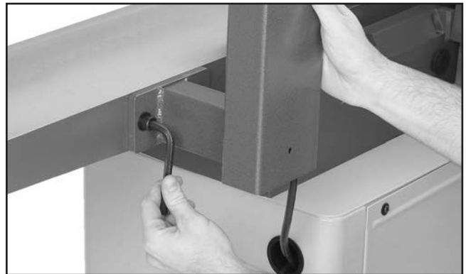
Figure 15. Attaching pedestal switch to stand.
