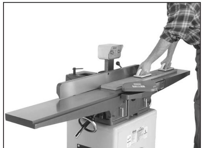
Figure 26. Typical surface planing operation.
