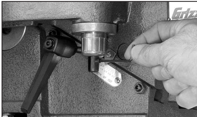
Figure 14. Example of installing cutterhead guard set screw.
