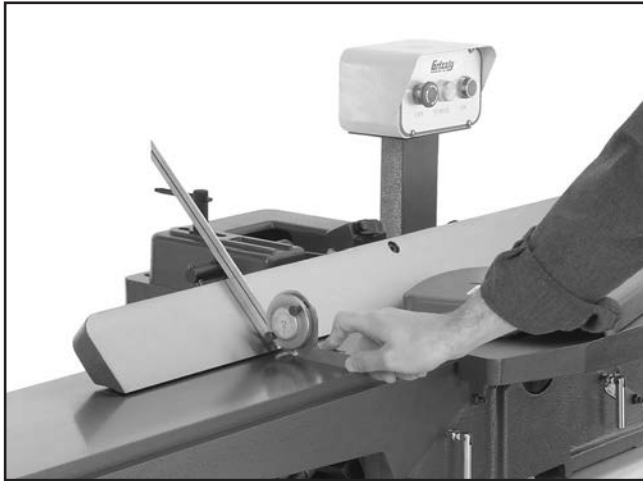
Figure 62. Example of adjusting fence 45° outward.
