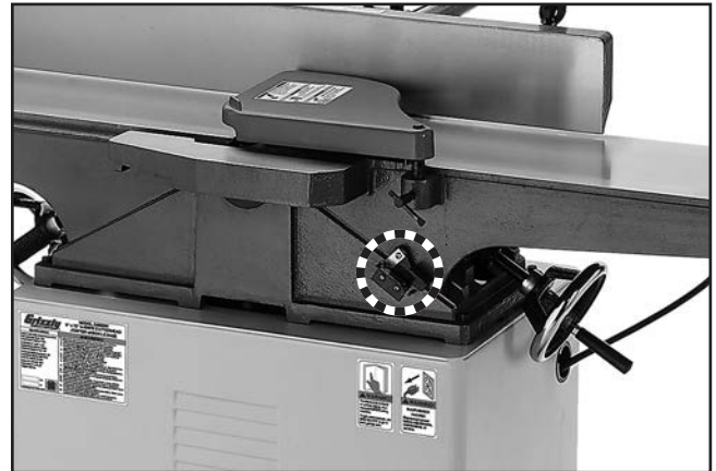
Figure 35. Location of depth-of-cut scale.
