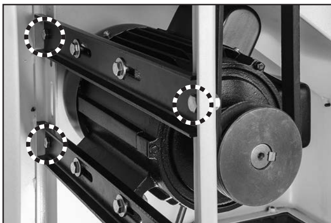
Figure 17. Location of motor mount bracket hex bolts/nuts (3 of 4 shown).
