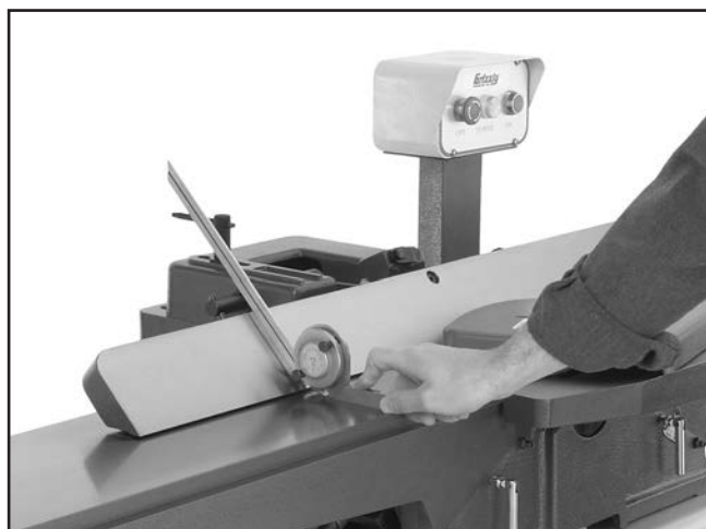
Figure 72. Example of adjusting fence 45° outward.
