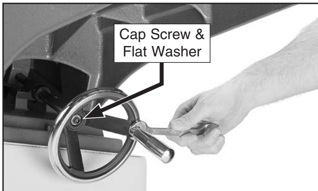
Figure 24. Securing the handwheel handle.
