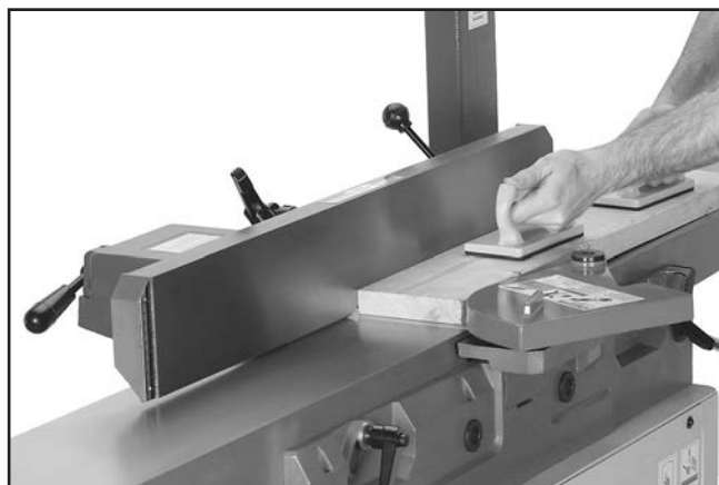
Figure 39. Example of surface planing operations.
