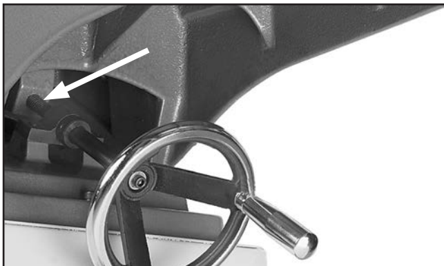
Figure 57. Leadscrew lubrication location.
