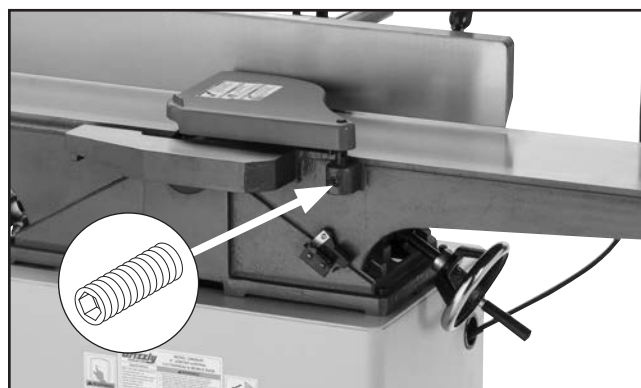
Figure 19. Cutterhead guard installed.
