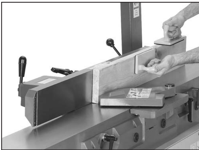
Figure 41. Example of edge jointing operation.
