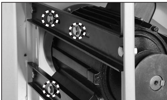
Figure 16. Location of motor mount hex bolts/nuts (3 of 4 shown).
