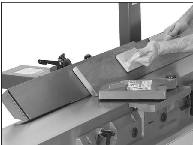
Figure 43. Fence setup for a bevel cut of 45°.
