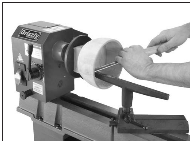
Figure 39. Typical faceplate turning operation.
