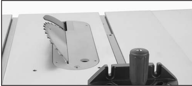
Figure 60. Blade tilted to 45° for bevel cutting on a typical table saw.
