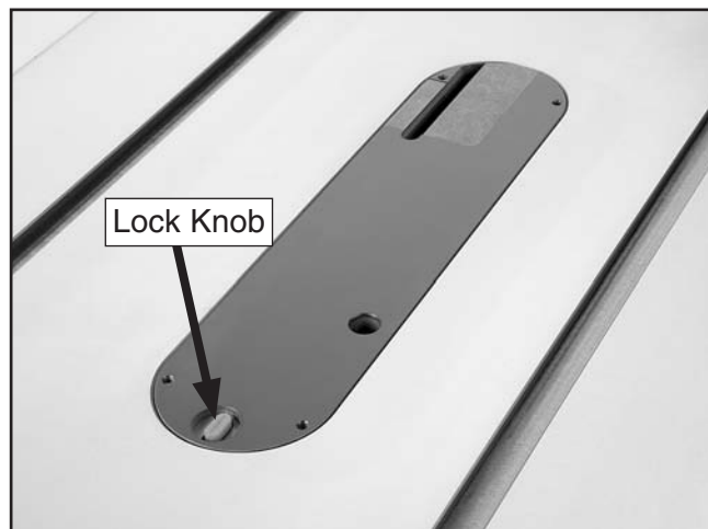
Figure 28. Example of insert lock knob unlocked.
