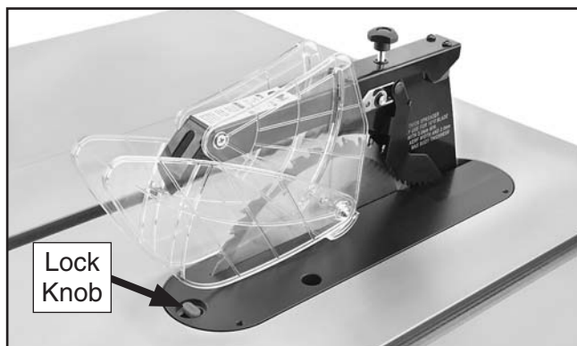
Figure 48. Blade guard and insert properly installed.
