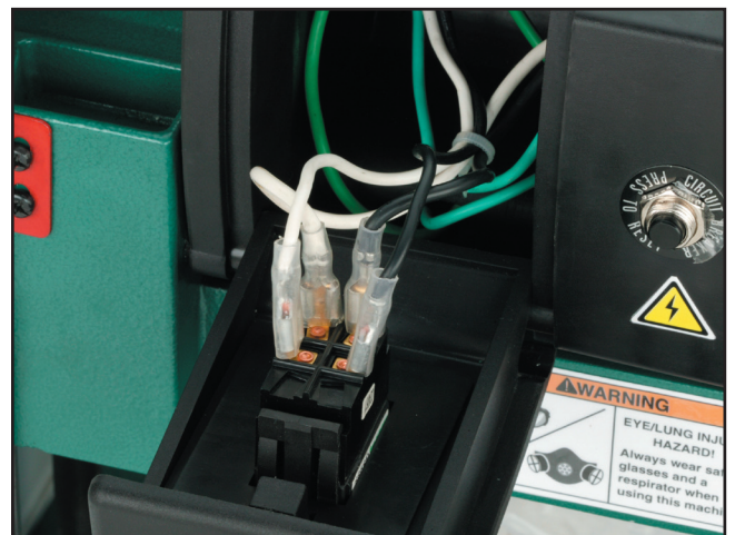
Figure 28. Switch wiring.
