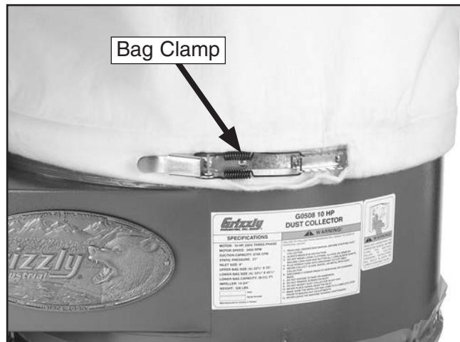
Figure 17. Upper filter bag secured to collector.
