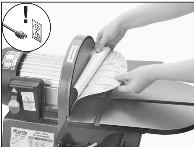
Figure 9. Sandpaper being slipped between the disc and table.
