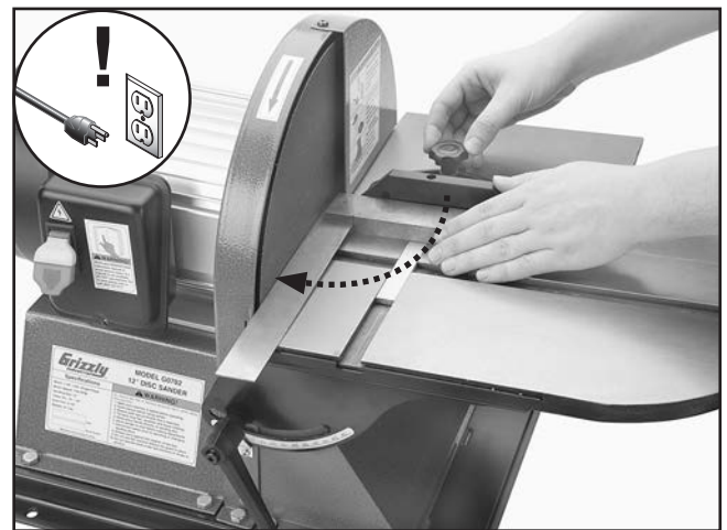
Figure 18. Squaring miter gauge to disc.
