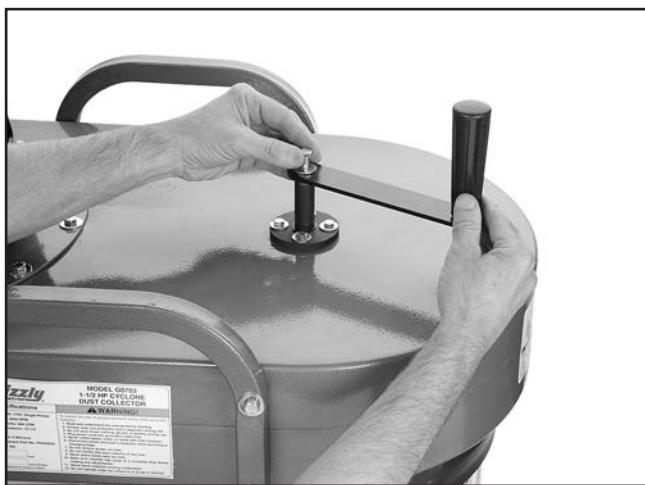
Figure 18. Hand crank installation.
