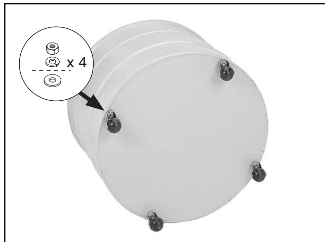
Figure 19. Dust collection drum casters installed.
