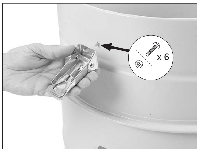
Figure 20. Lid latch installation.
