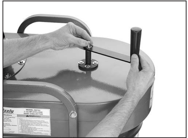
Figure 9. Installing hand crank.
