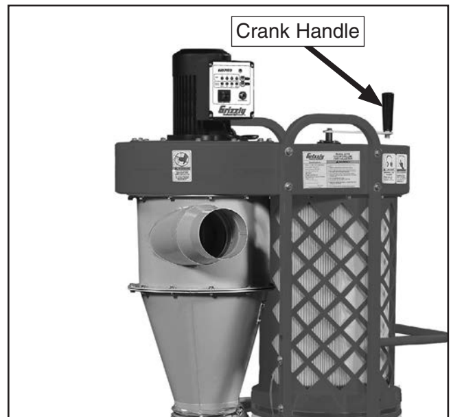
Figure 63. Brush handles for cleaning canister filters.
