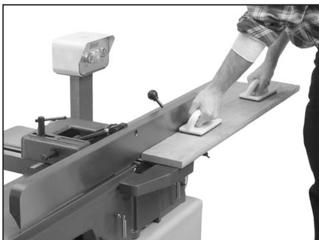
Figure 31. Typical rabbet cutting operation.
