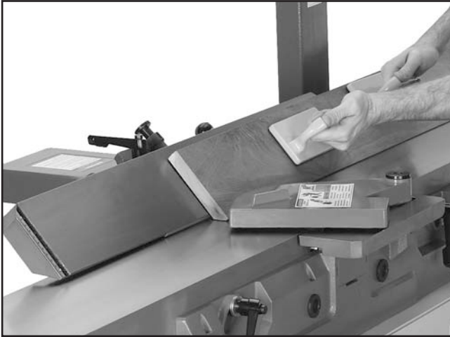
Figure 29. Fence setup for a bevel cut of 45°.
