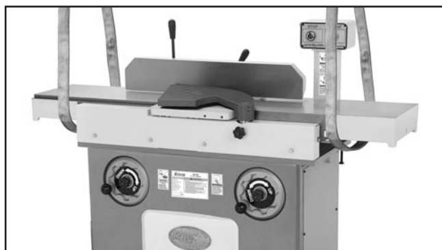
Figure 7. Model G0706 supported evenly by two lifting straps.
