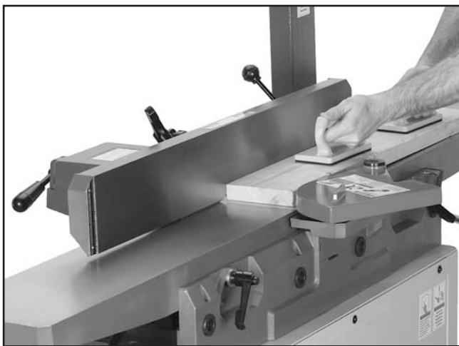
Figure 25. Example of surface planing with the jointer.
