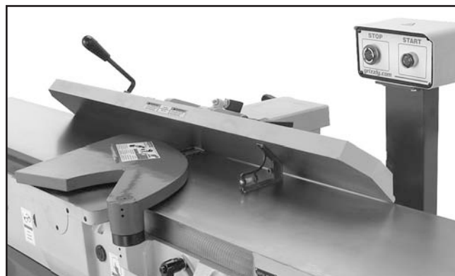
Figure 60. Fence adjusted 45° inward.
