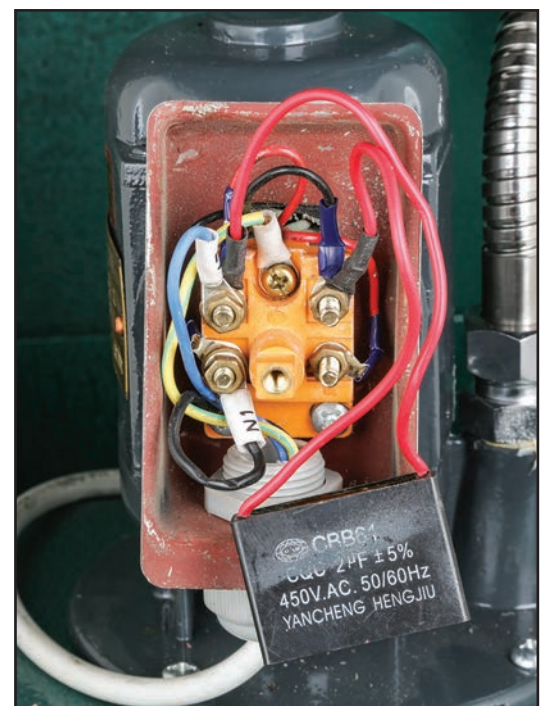
Figure 144. Coolant pump wiring.
