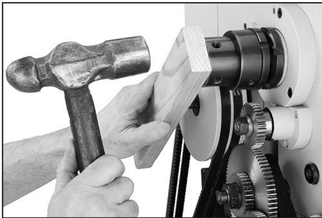
Figure 136. Example of unseating spindle bearings to introduce spindle end-play.
