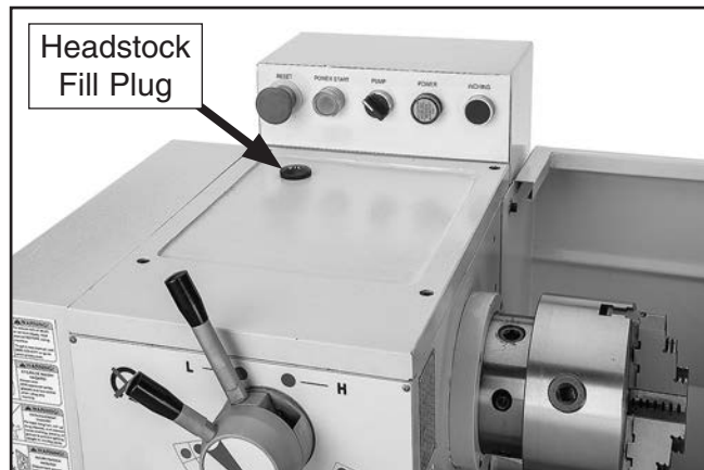
Figure 109. Location of headstock fill plug.
