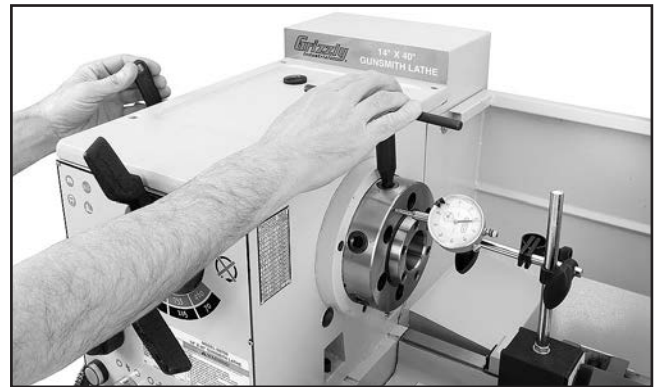
Figure 138. Example of adjusting spindle bearing preload.
